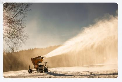
The HKD Diablo is the workhorse in our fan line up. The Diablo is engineered for simplicity and efficiency and is capable of water flow up to 250 GPM with projection exceeding 225 feet.
