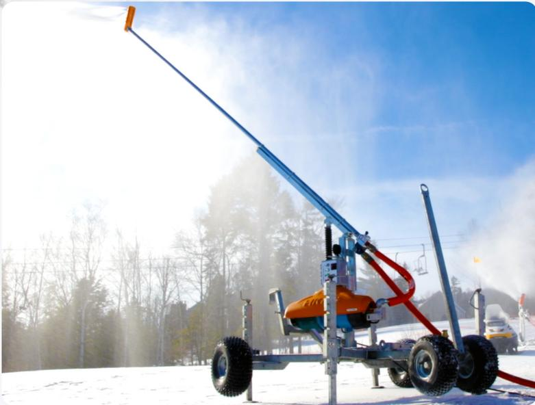
The HKD Volt is the “airless” low energy workhorse in our tower gun line up. The Volt incorporates our SV14 snowgun design and Rotary Valve Technology allowing 5 water flows.
