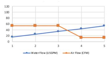
Nozzle configuration and flows can be customized based on user's climate and snowmaking objective.
